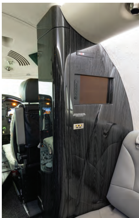
Duncan Aviation uses a process called hydrodipping to expand cabin design options while reducing cost and downtime.
